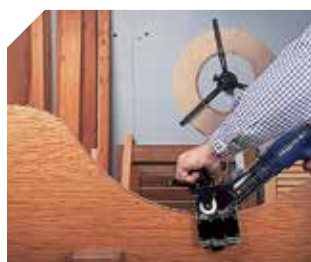
Possibility to band straight, circular or shaped pieces.
