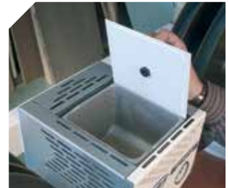
Easy access glue tank on top. The glue application system includes an easy, non-stick silicon roller.
