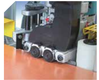
Simultaneous top and bottom trimming, with radius or 10° chanfer. Flat scrapers after the trimming unit.
