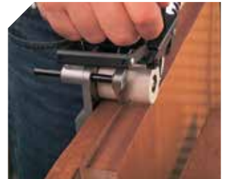
Banding the upper side of the lap.
