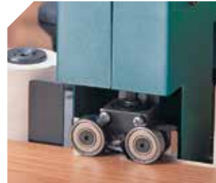
Power trimming unit: trimming both sides simultaneously.
