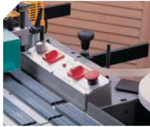
Safety control (STOP). Electronic temperature control.
