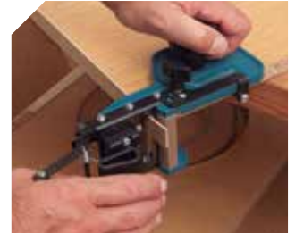
Cutting on both sides on straight panels.
