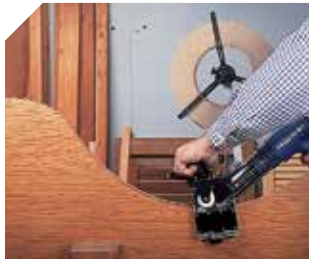
Enables banding of circular or shaped pieces.
