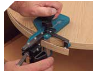
Cutting on circular panels.
