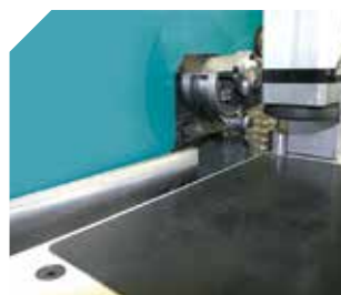
Guiding fence on the side of the tape to be trimmed.
