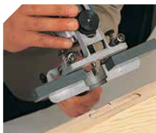
Placing hinges with the ZB93 head.
