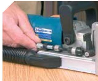
Quick adjustment of different slotting depths.
