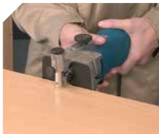
Excellent finishing when trimming laminates.
