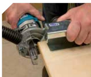
Optional accessory (5646343): Precise guiding for corner trimming.
