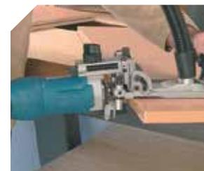
Trimming the edge with the straight bit.
